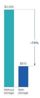
$<sup>^1</sup>$  kW = kilowatts. Load-profile assumptions are: station has 4 direct-current fast-charging 50 kW chargers; 11 charging sessions occur during time period profiled (4:00 a.m. to 7:00 p.m.); in at least 1 instance, 2 cars charge simultaneously; demand-charge rate is \$30 per kW; and battery-storage system is 150 kWh and can discharge at up to 75 kW.
